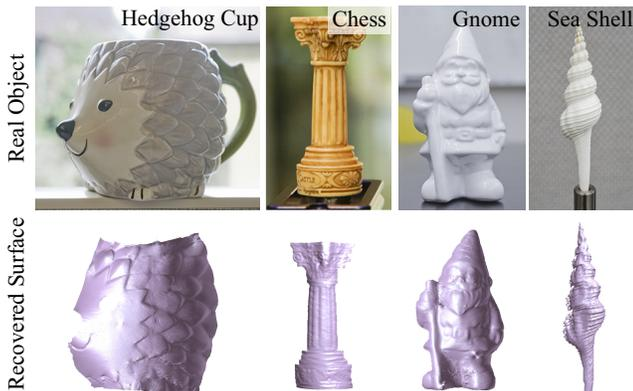
Figure 10. Surface reconstruction results.
